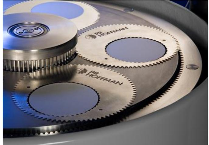
The top plate downforce is controlled by a servo driven ball screw. The controller constantly adjusts the downforce based on feedback from a load cell that is mounted on the top plate drive shaft. This control loop allows precise control of downforce on the parts. The lapping force range is from 15 to 275 pounds [6.8 to 125 Kg]. Changes to the downforce are made gradually through the servo motor. This same motor is used to raise and lower the top plate.
