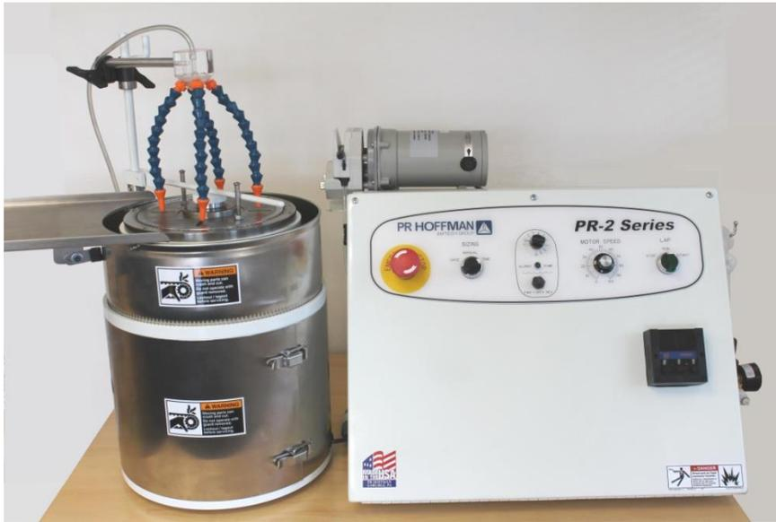
The P.R. Hoffman PR-2 Series lapping and polishing machine is a small table top machine designed for finishing a variety of small parts with excellent results. It is ideal for research and development applications where small quantities of parts are common. The pieces to be processed are placed in carriers (work
