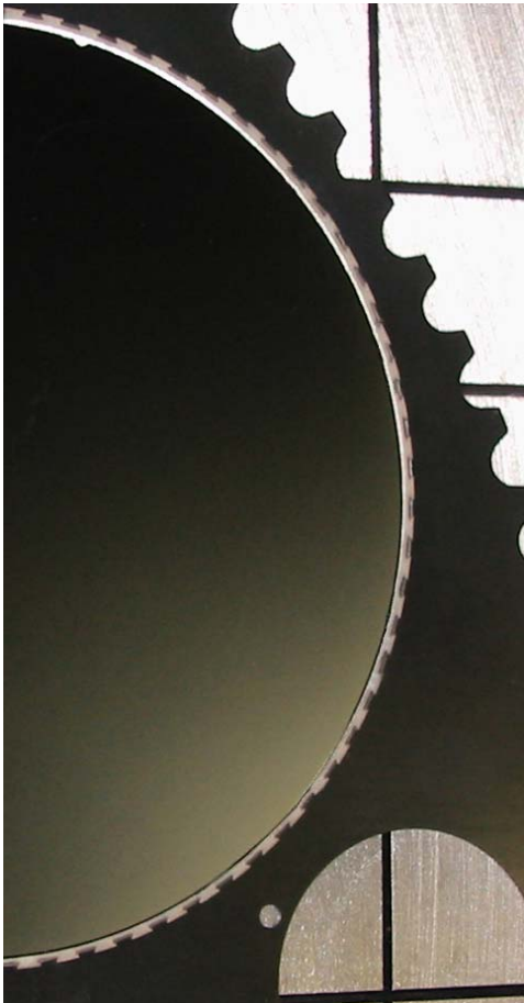
Photograph of 200 mm Insert Carrier and silicon wafer.
